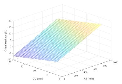
**Figure 4**. Influence of rotor speed (RS) and concave clearance (CC) on grain breakage (GB)
