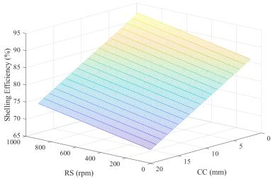
Figure 3. Influence of rotor speed (RS) and concave clearance (CC) on shelling efficiency (SE)
